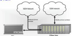
PRImaGate Switch is able to analyse dialled number and forward the call trough GSM Network or PSTN PRI access. Also, if all GSM modules are busy, it is possible to forward the call trough PSTN PRI network. Calls coming trough PSTN PRI access are forwarded directly to the PBX.
